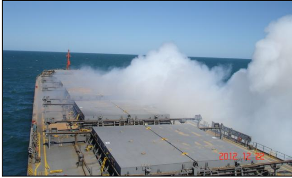
Figure 4: Smoke from cargo hold hatch no. 4
