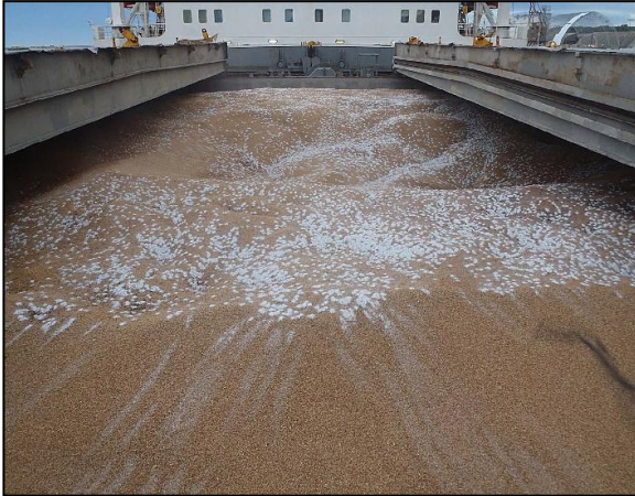
Figure 7: Aluminium phosphide tablets distribution in cargo hold no. 2
