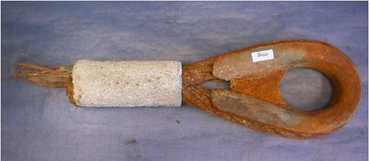
Figure 9: The fractured steel wire Source: FORCE Technology
