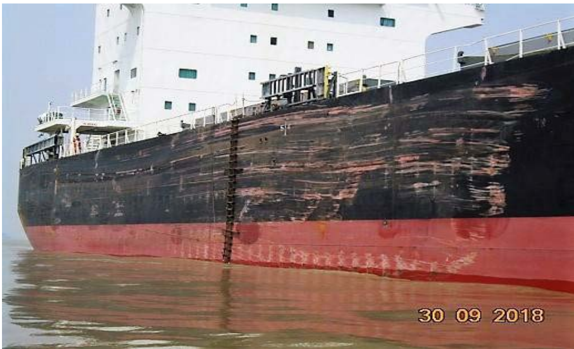
FIGURE 8 – Allision Damage to the NEW LEGACY
