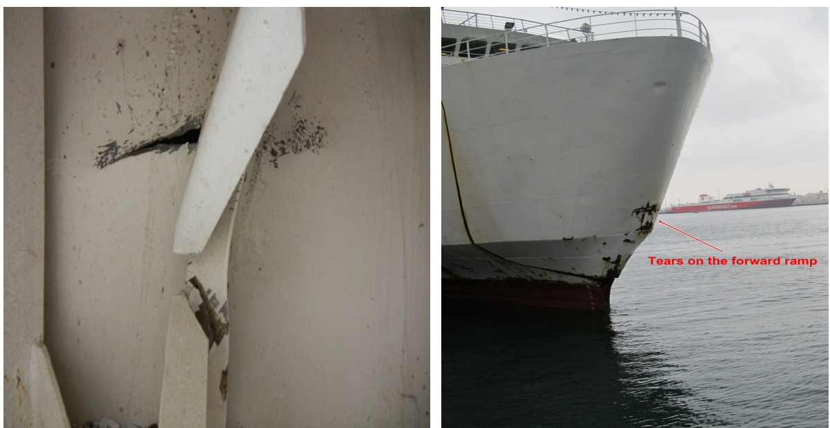
Figure 9: Damage to the bow of ANKARA (1)
