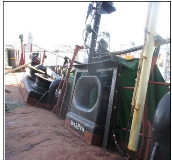
Figure 9: Deformations on poop deck
