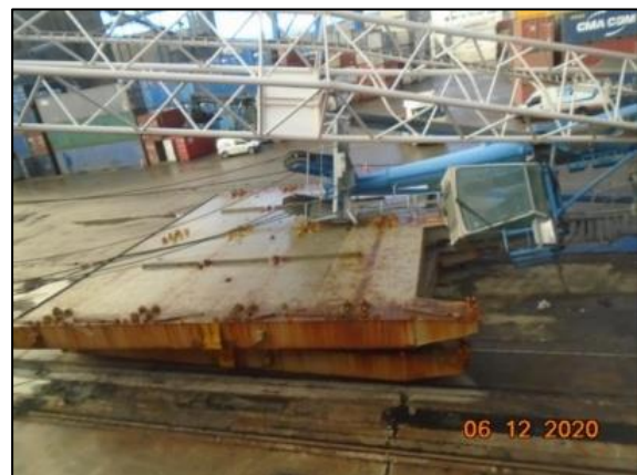
Figure 6: The hatch covers of bay 10 struck by the mobile shore crane
