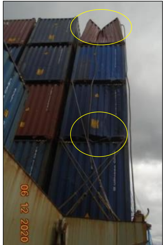
Figure 5: Several damages sustained by the containers on board Atlantic North
