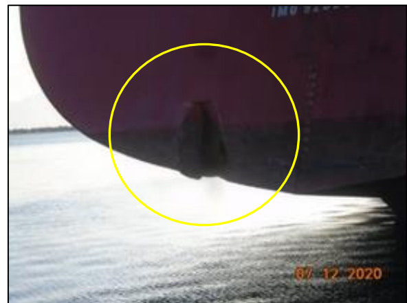
Figure 2: Hole in aft peak tank
