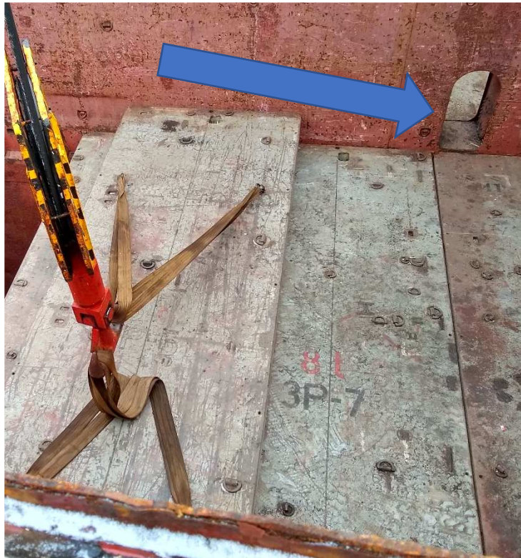
Figure 5 - Manhole between PS and SB cargo hold
