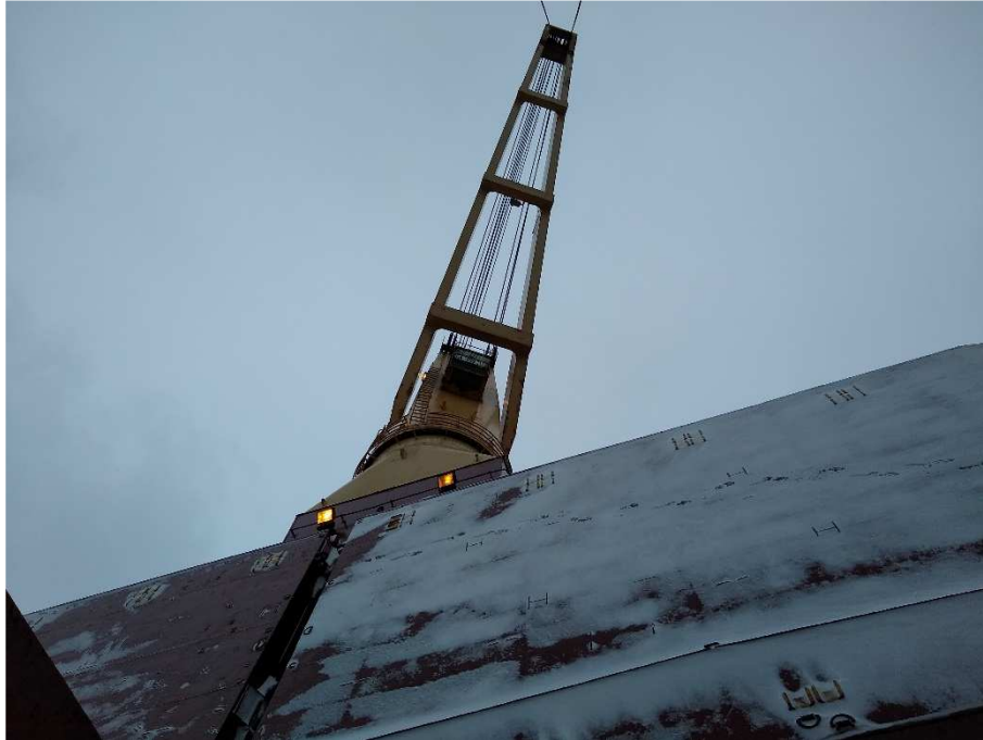
Figure 2 - Deck crane used for shifting pontoons.
