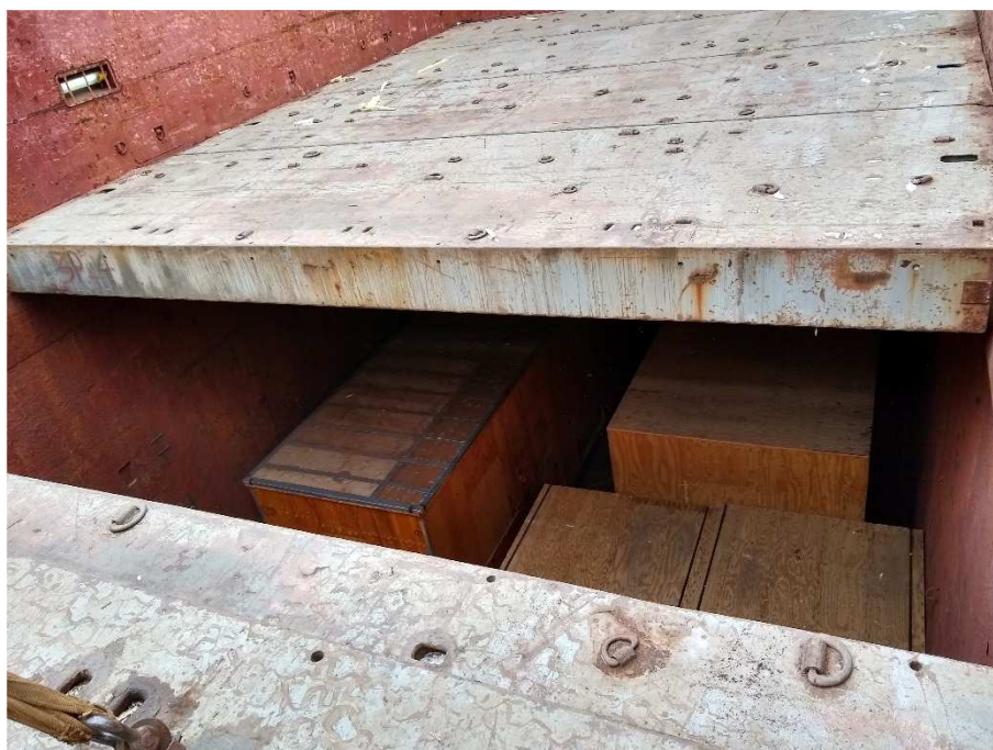
Figure 1 - Cargo below the tween-deck pontoons in cargo hold 3 PS
