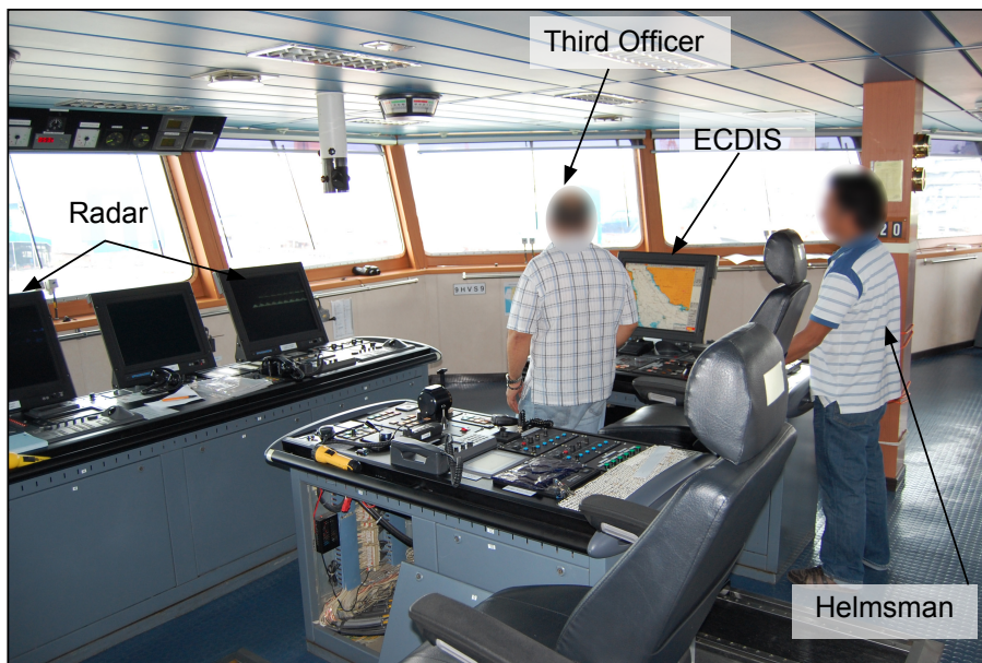
Figure 2: View of ECDIS and position of bridge team
