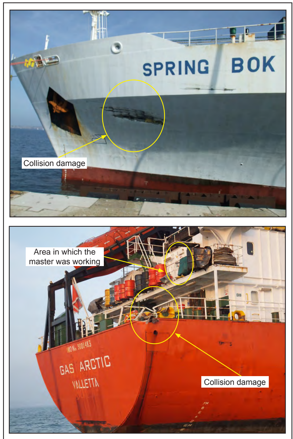
Figure 6: Damage to both vessels
