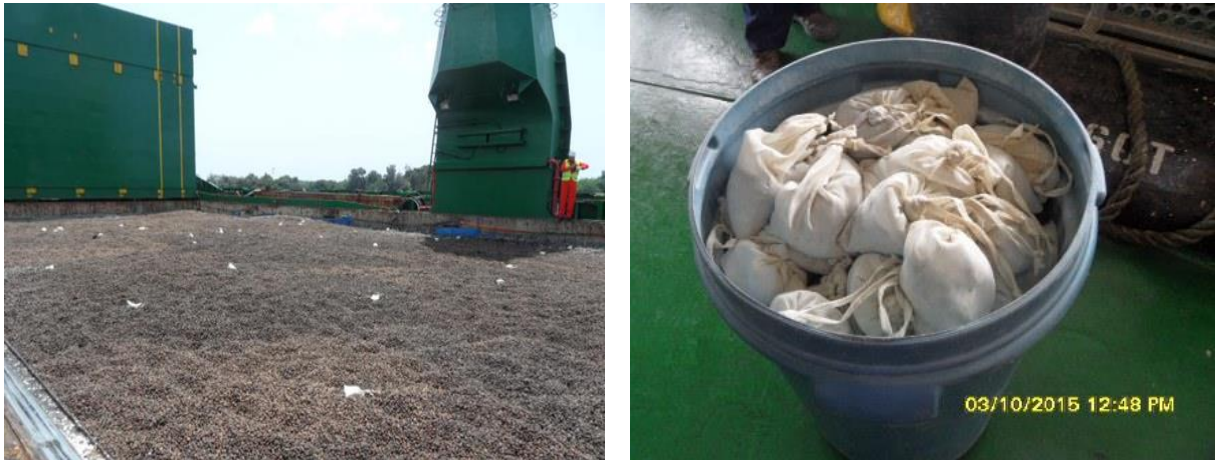
Photograph 4. Phosmium bags distributed on top of cargo and placed in a container after the accident, at San Pedro.
