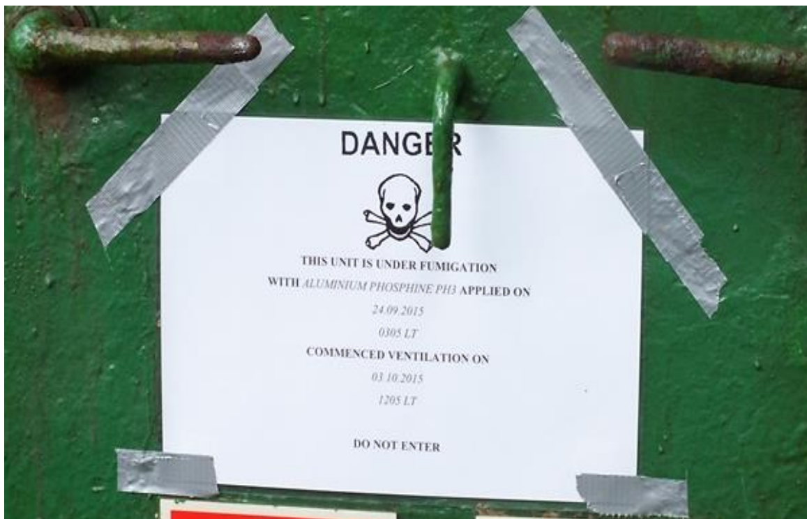
Photograph 9. Entry to the Nefryt cargo hold marked during ventilation with a sign warning of fumigation using PH 3 .
