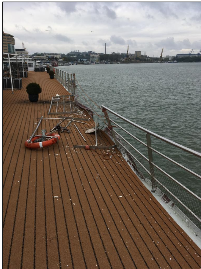
Figure 5.8 – Damages to upper deck
