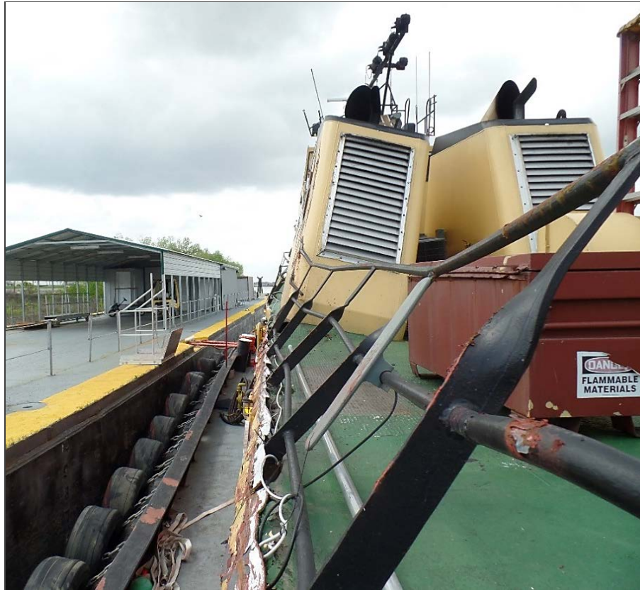
Port side of the Texas , showing bent handrails and damaged stack. (Photo by the Coast Guard)
