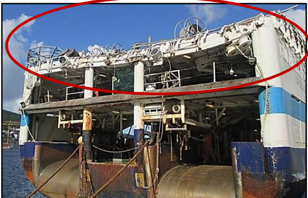
Damages on the after part of the upper deck of PRINCESS, alongside at berth Jekteviken 1 after the collision - credit GeofieLD.
