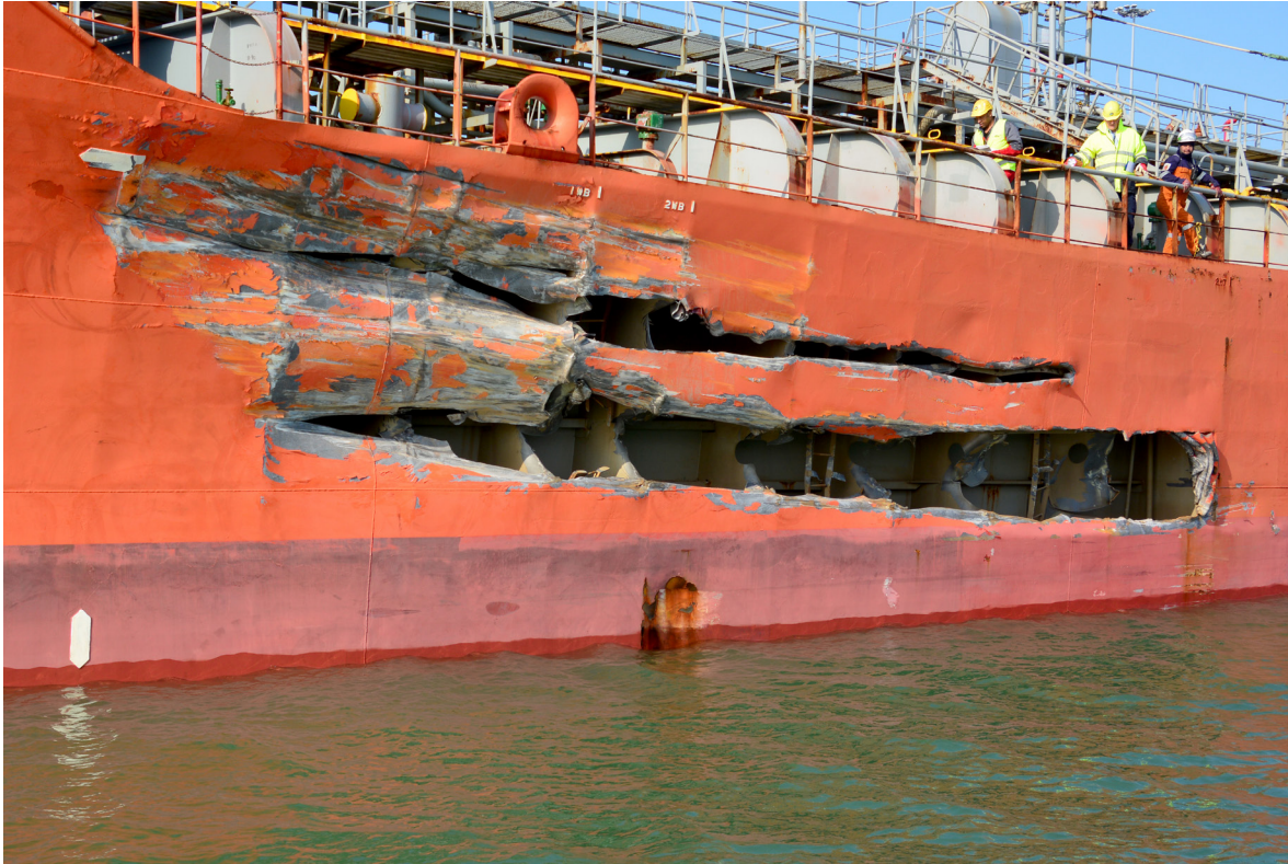
Figure 8: The damage to the Chemical Marketer following the collision with the Viking Idun.
