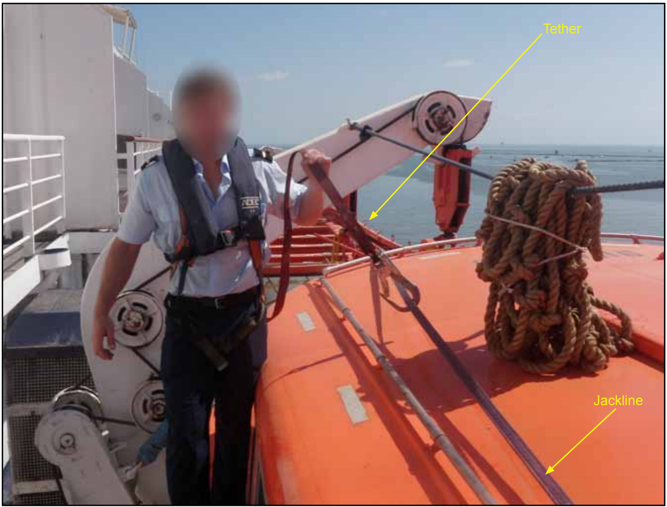
Figure 21: Saga Ruby's tender jackline and tether arrangement
