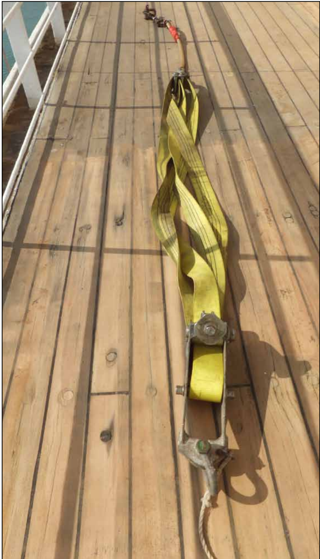
Figure 18: Wire, strap and ratchet bowsing tackle
