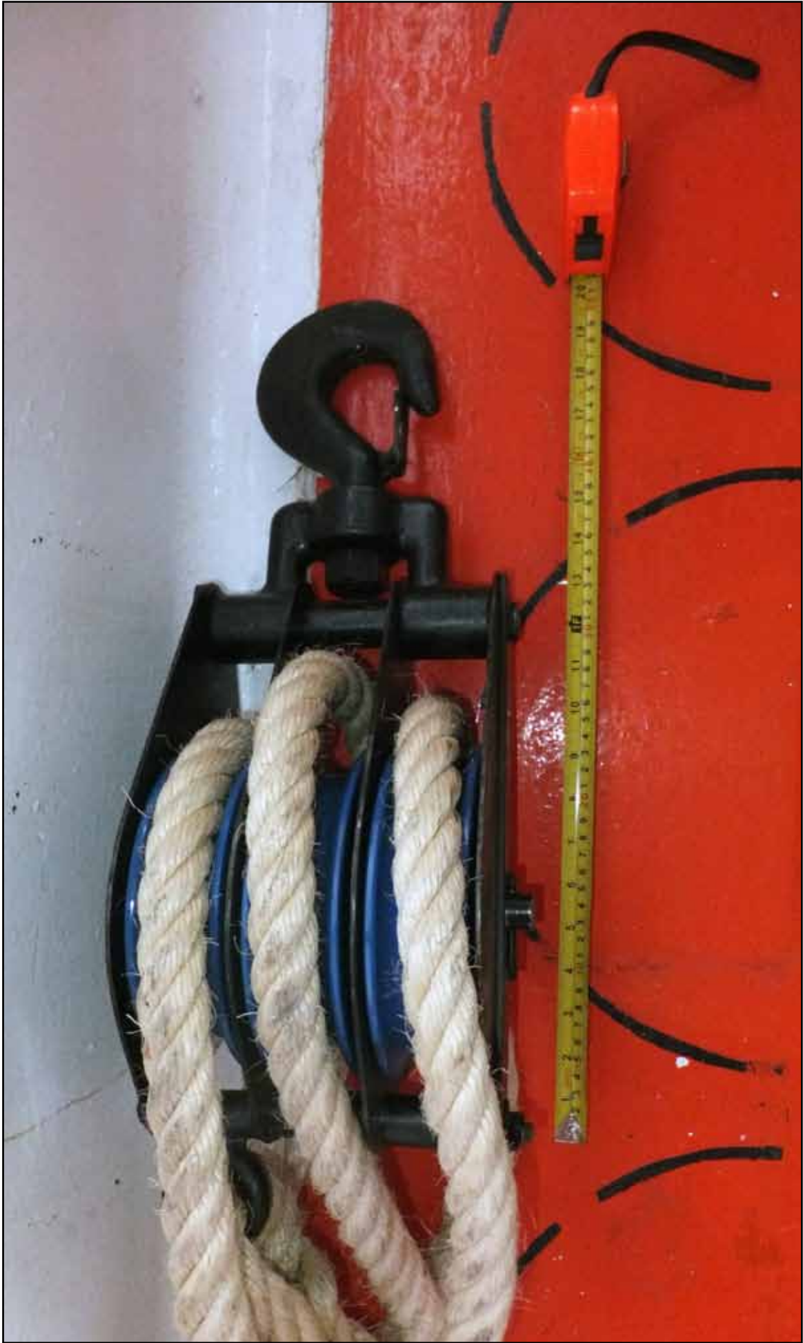
Figure 19: Three-fold bowing tackle block
