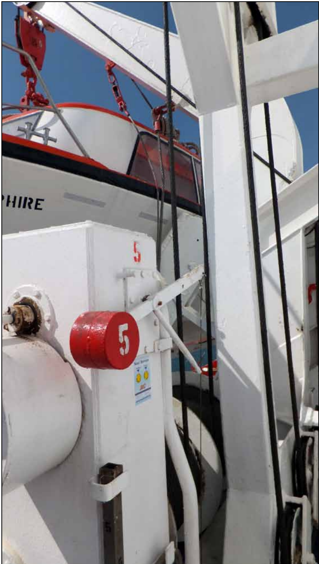
Figure 10: Davit control position on the winch deck
