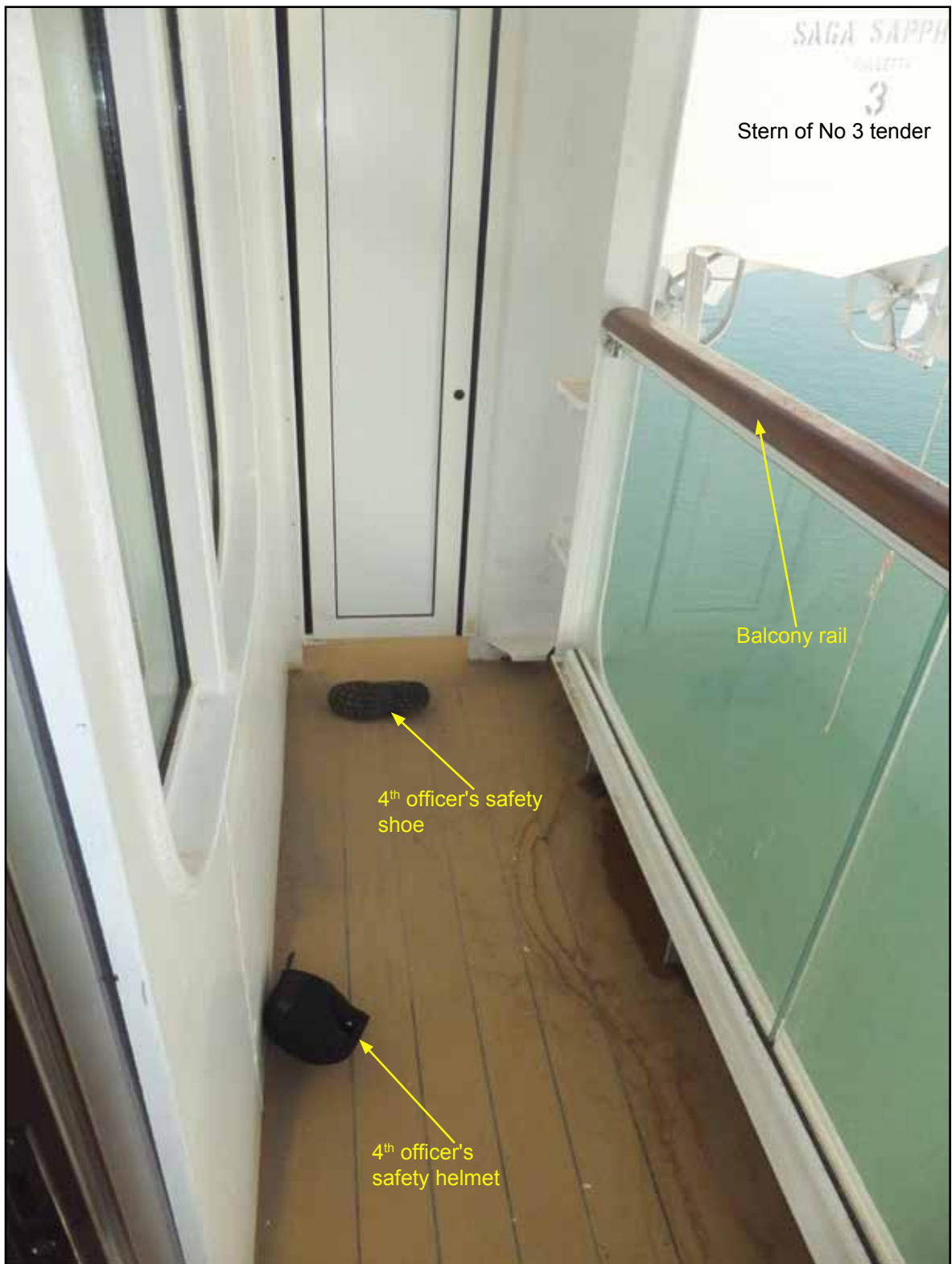
Figure 8: Balcony rail of cabin 8036
