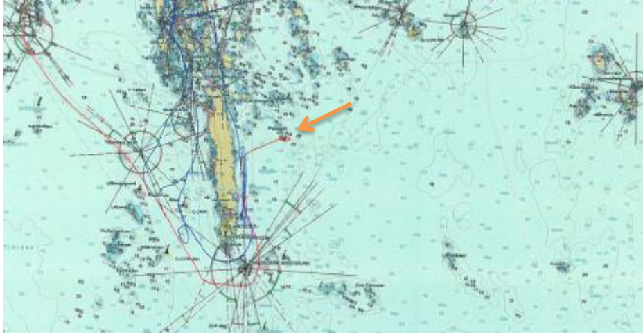
Figure 2. The area around Landsort. The red track is KERTU's. The blue track is the pilot boat's. The arrow mark the position of the grounding. The islands to the right in the image are Gunnarstenarna.
