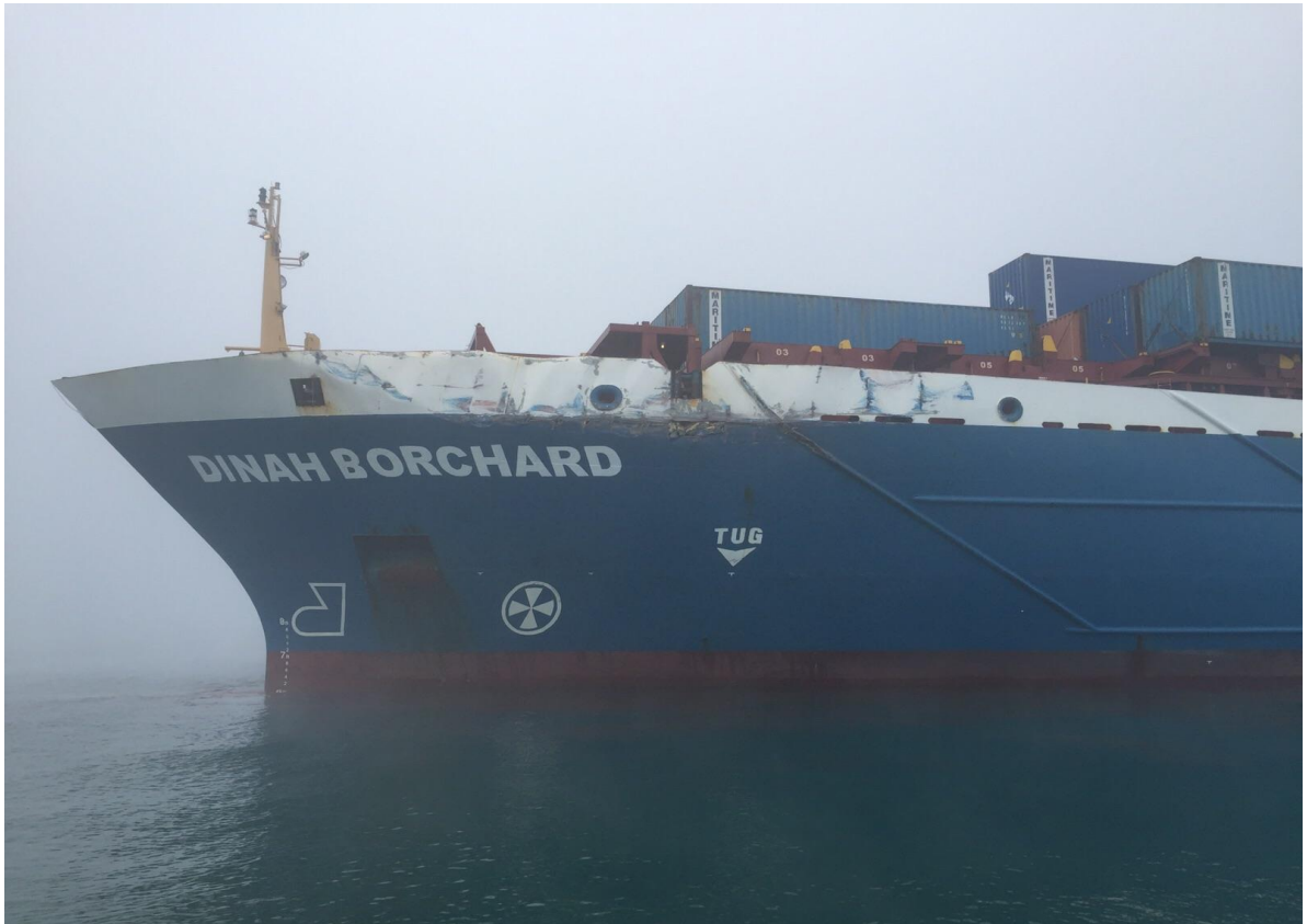
Figure 5: M/V "Dinah Borchard" Port side shell plating deformed ( i.w.o. rope store, bosun store, paint store at connection to main deck with one crack at frame 162, and two small ones frames 174-175 and 171-172)
