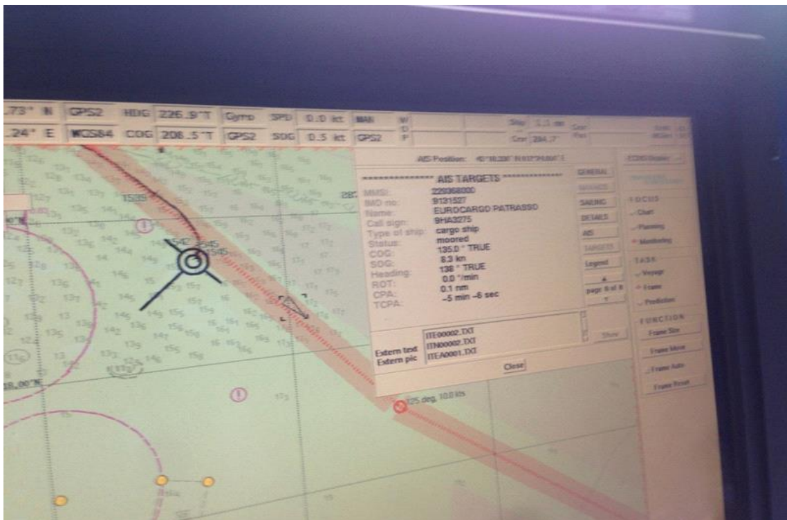
Figure 4: M/V “Dinah Borchard” ECDIS&AIS display (after collision, AIS target EUROCARGO PATRASSO moored)
