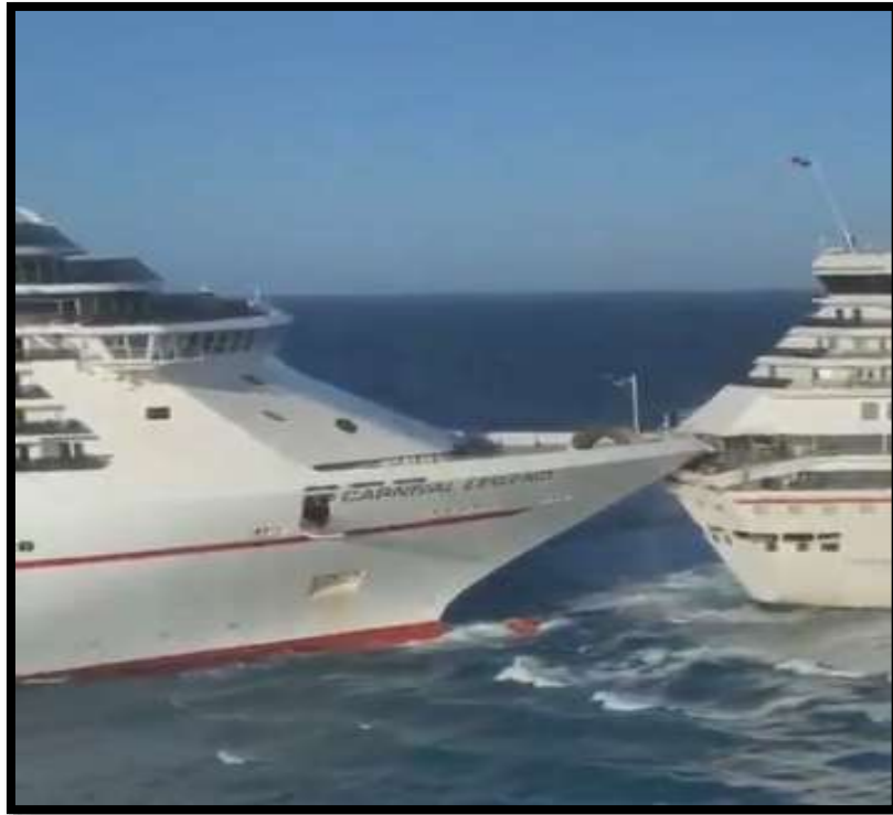
Figure 3.2: Affected area of Carnival Legend (suffer minor's structural damage on the bow (portside)).
