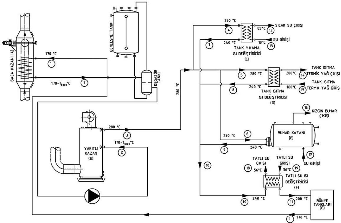
*Line Diagram 2 Similar Thermal Oil Boiler Line Diagram*
