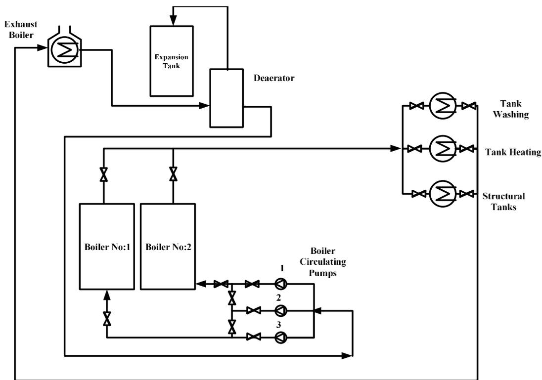
*Line Diagram 1 Boiler Line Diagram of the M/T TORC (Concept)*
