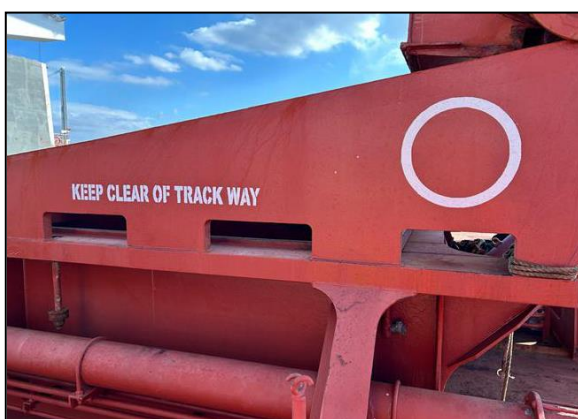
Figure 6: One of the warning signs at the cargo hold's hatch cover trackway
