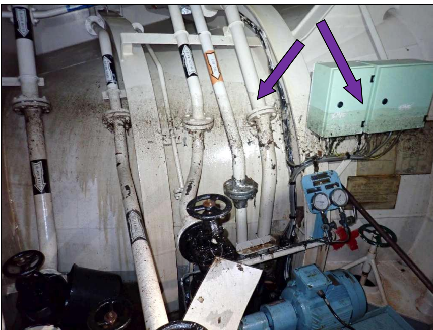
Figure 5: High water marks in the engine-room following completion of the pumping operation
